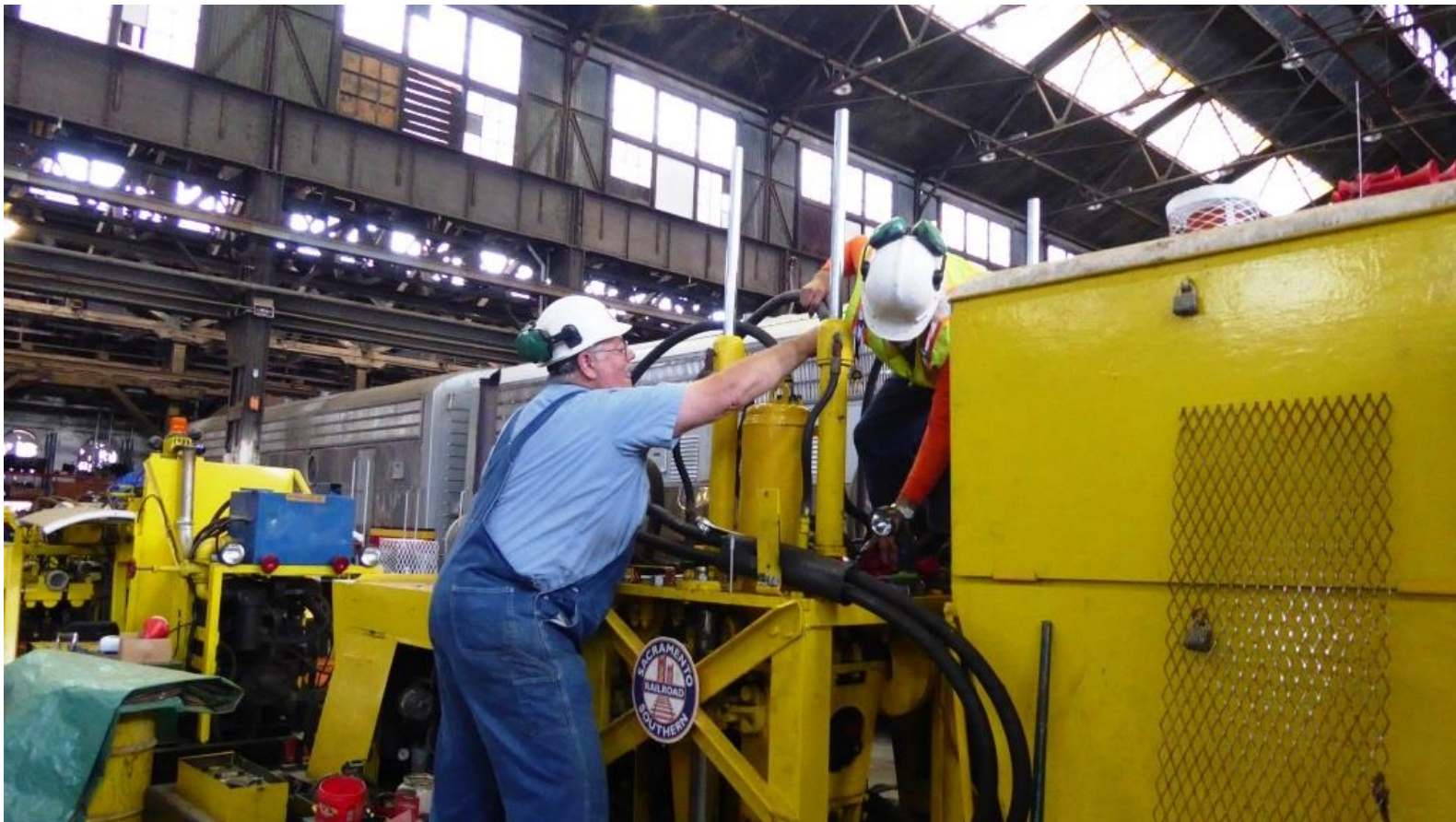
Meanwhile, Chris and Ed re-plumb the tie-shear
